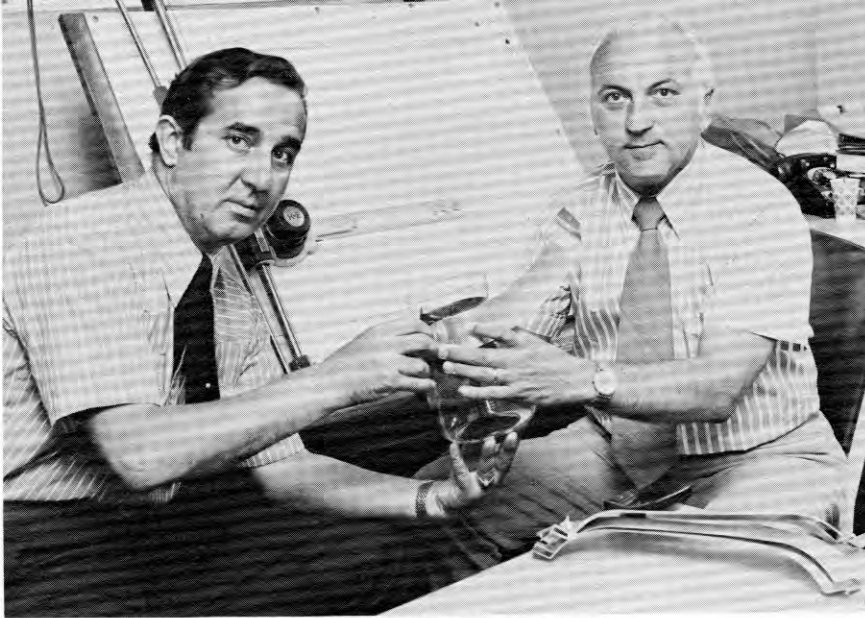
Kurt Kopf, left and Richard Miller inspect percolator bands which are made of .024" thick aluminum on a No. 6 Minster OBI.
