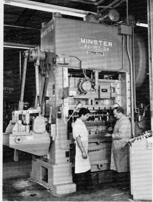
Highly automated P2-150-54 press in Buhrke plant.
