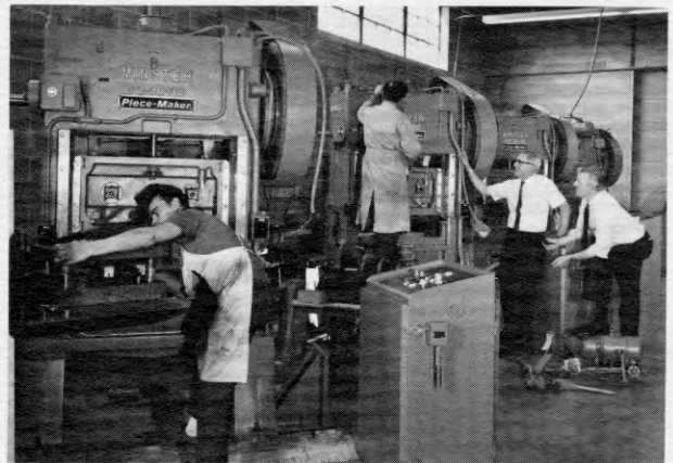
Minster P2-30 Presses to manufacture ring pull tabs for the can industry.
