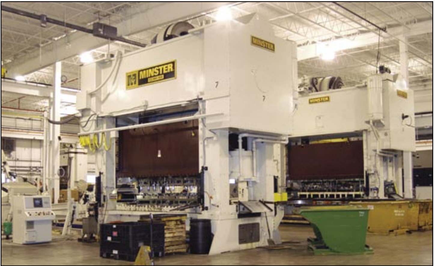
Two New Minster E2-800 ton press equipped with Alternative Slide Motion (ASM) have increased the manufacturing capacities and capabilities at Destiny Manufacturing.
