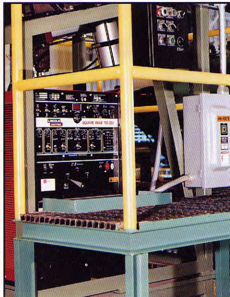
The high quality lamination seam (top) produced by the coil end joiner using a Lincoln Electric Square Wave TIG 355 welder (right) assures there is no interruption to production flow.
