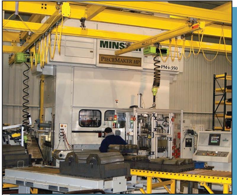
***Minster PM4 press producing stacks of laminations at the Lincoln Electric Company.***
