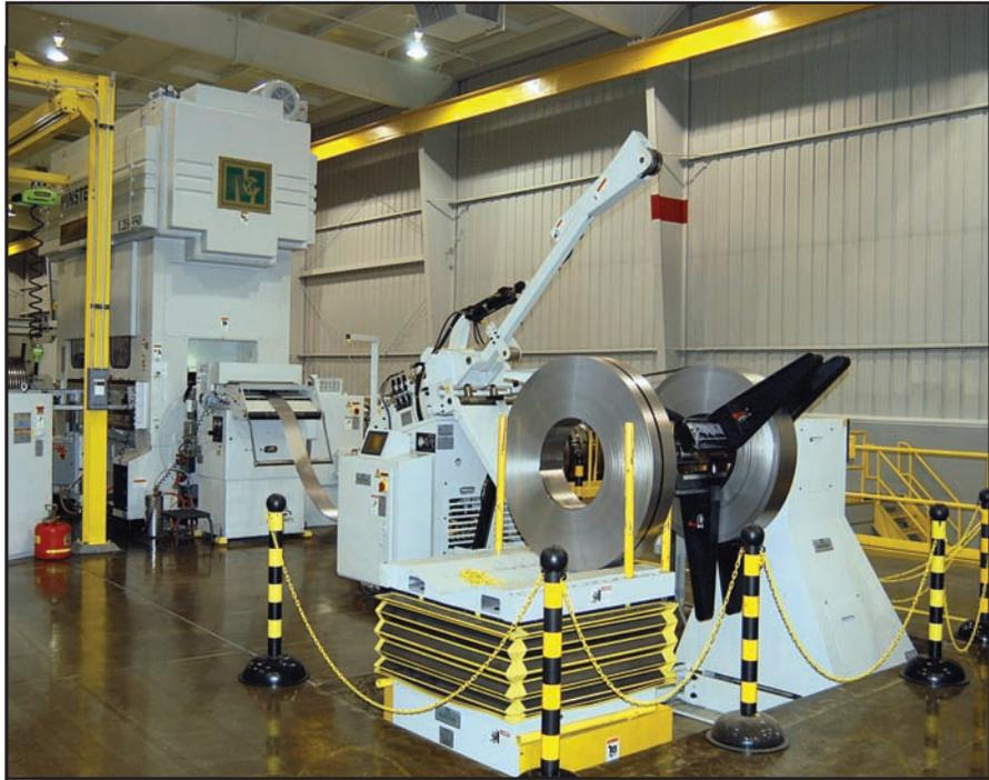
***E2H 350 press at Lincoln Electric includes a complete and integrated Minster Coil Line.***
