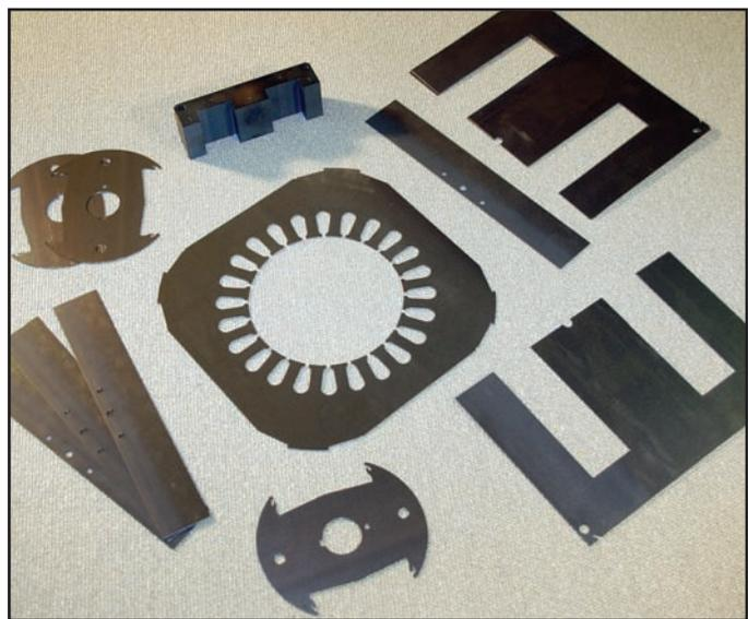
*Some of the many types of laminations produced by Lincoln Electric for use in the company's welding products.*
