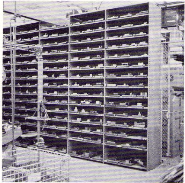
All Die-Namic dies are neatly and conveniently stored a few feet from the press. Die changes are done very quickly.
