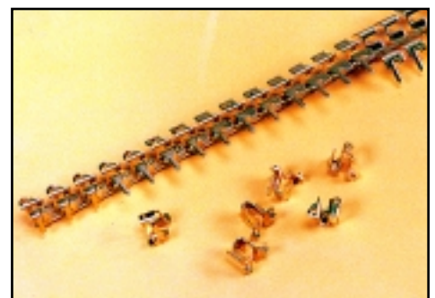
Sample of the variety of parts produced on Minster presses at Norwood Tool.
