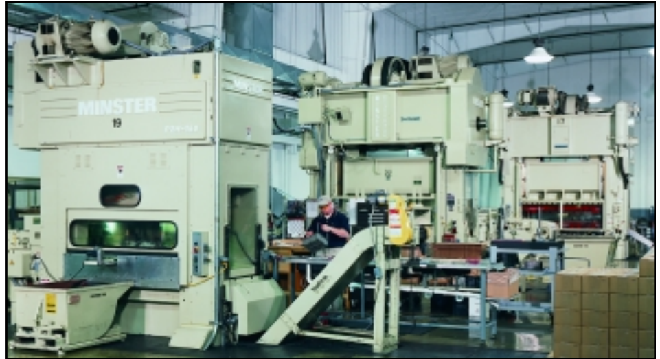
Norwood Tool continues to expand its progressive die stamping capabilities with the addition of Minster P2H and E2 presses.
