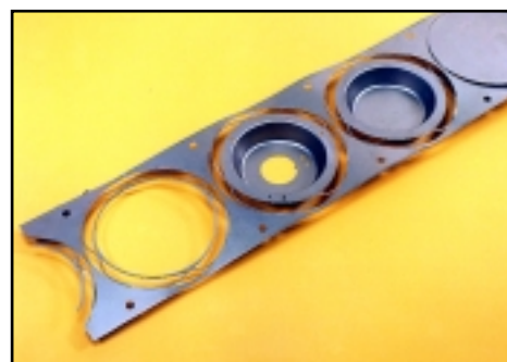
Sample of the variety of parts produced on Minster presses at Norwood Tool.
