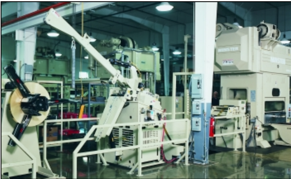
This Minster P2H press at Norwood Tool is equipped with a Minster Reel, Straightener, Thread Table and Feed. The line is integrated with the press via Minster's Production Management Control.
