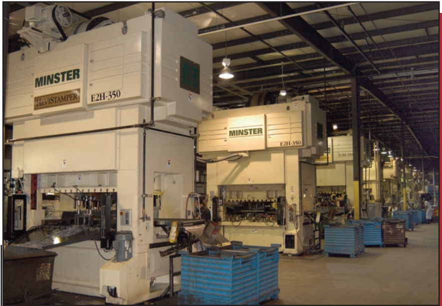
Located in Slatillo, Mississippi, Omega Motion's manufacturing capabilities include three Minster E2H-350 presses.
