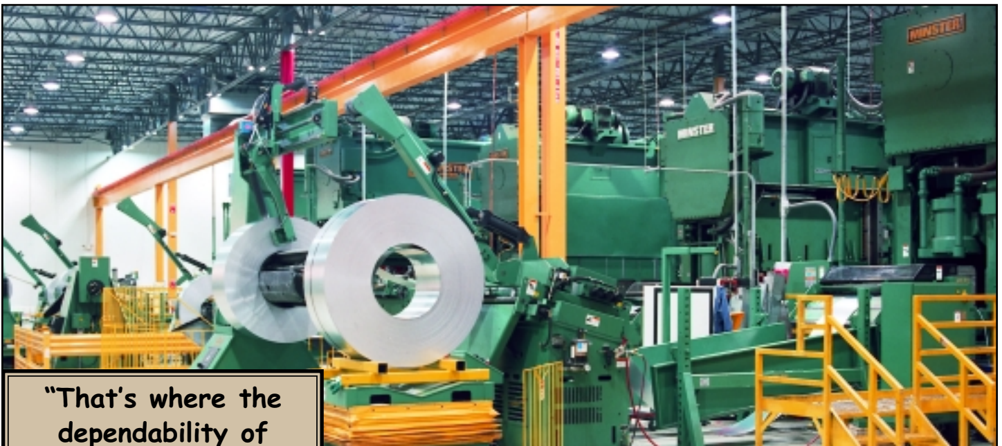
Several Minster presses and coil lines aid in the production of computer components at Trend Technologies.
