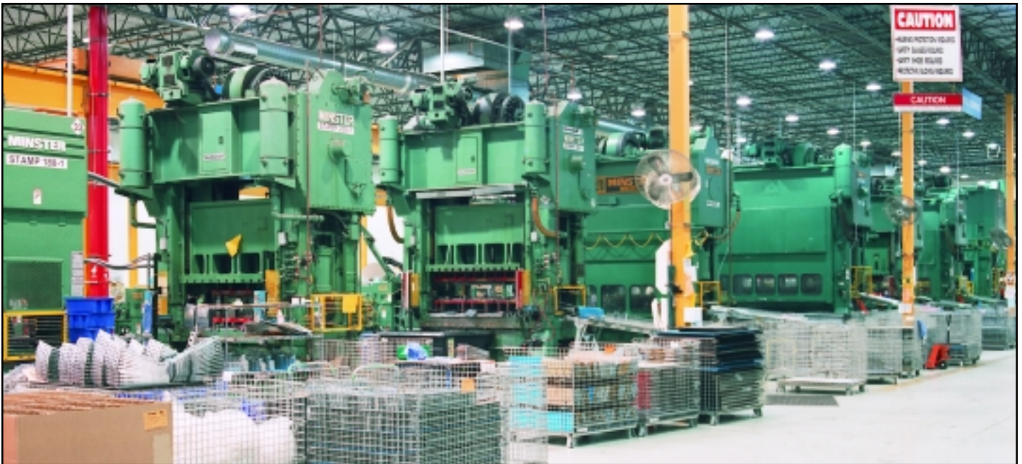
Several Minster presses and coil lines aid in the production of computer components at Trend Technologies.
