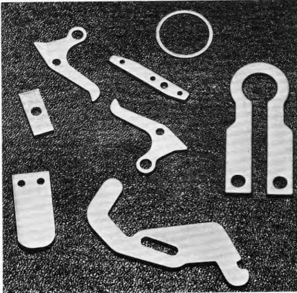
Typical parts for Westinghouse electrical products made with Die-Namic Process.
