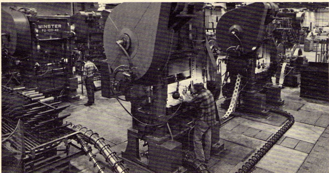
View from back side of a tandem press line shows how laminations flow through chutes from presses to unloading station.
